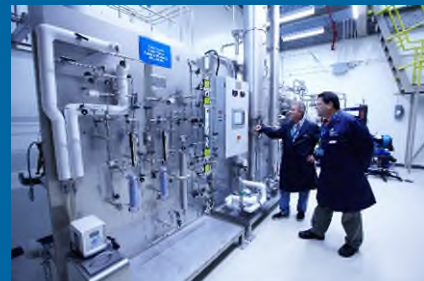
Top - Operator adjusting conditions for High Temperature Steam Electrolysis materials development for hydrogen production. (Source: CNL)
